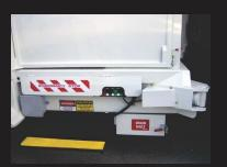
Hopper steps with integrated safety pads to interrupt power.
