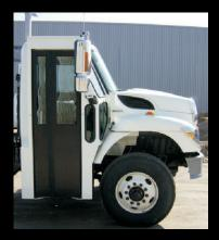
Automated bifold doors open with work-brake and close when operator returns to cab.
