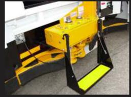
Hopper steps with integrated safety pads to interrupt power to the arm.
